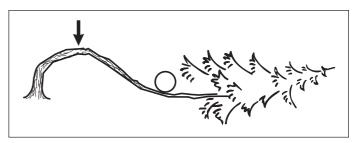
b) Decide which is the SAFEST way to release the tension and whether YOU are able to do it safely. In complicated situations the only safe method is to put aside your chain saw and use a winch.
